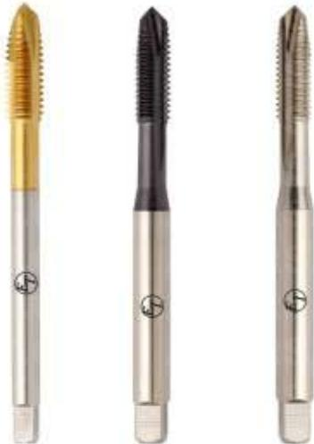
Emkay Tools specializes in application taps for various applications. Spiral Point Tap Or Gun Nose Tap with 3-4 threads chamfer is recommended for tapping in THROUGH HOLES. These taps normally push the chips down the hole and are suitable for materials like aluminium, stainless steel, general purpose steel, forged steel etc.
